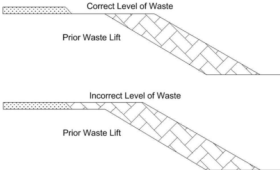
**Figure 12: Maintain correct waste floor level.**
