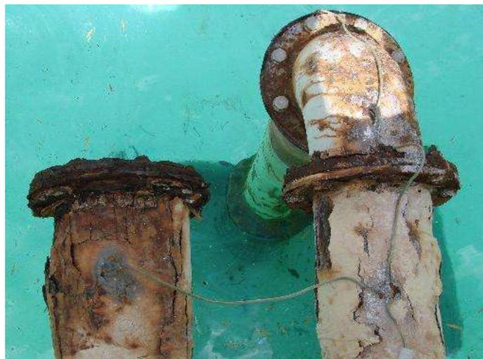
SCREENED FOOT VALVE AND PIPES TO BE URGENTLY REPLACED
