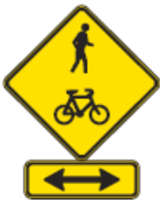
Figure 7: Bicycle/Pedestrian Warning Sign - AS 1742.9 W6-9 and W8-23
