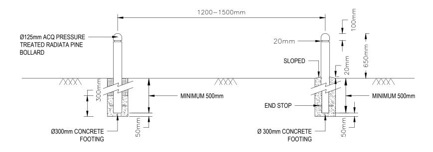
TYPE "A" - PARTIAL DEPTH CONCRETE FOOTING
